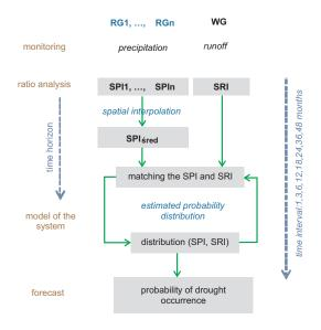
**Fig. 5.** Diagram of drought assessment, taking into account meteorological and hydrological conditions
